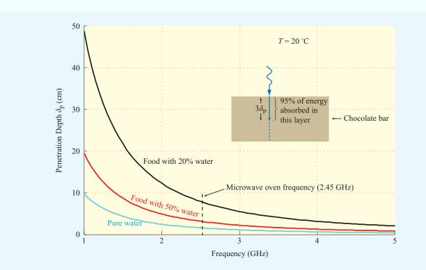
This is a practical range for cooking food in a microwave oven; at much lower frequencies, the food is not a good absorber of energy (in addition to the fact that the design
