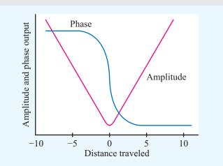
**Figure TF11-2** Amplitude and phase responses as a function of the distance by which the magnetic core is moved away from the center position.
